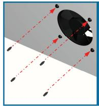
The specially developed safety rivets can be plugged-into the drilled holes of the fan sleeve pegs.
